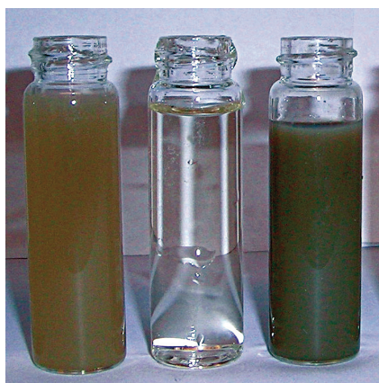
FIGURE 12.4. Water samples from plots with winter wheat from rainfall event (16 Sept. – Oct. 5) in 2004. Sowing date for winter wheat was 10 September. Left bottle; Autumn harrowed plot, SS – 1100 mg/l, Middle bottle, Direct Drilling plot SS – 5 mg/l and Right bottle: Autumn ploughing plot SS – 5820 mg/l, SS = suspended solids
