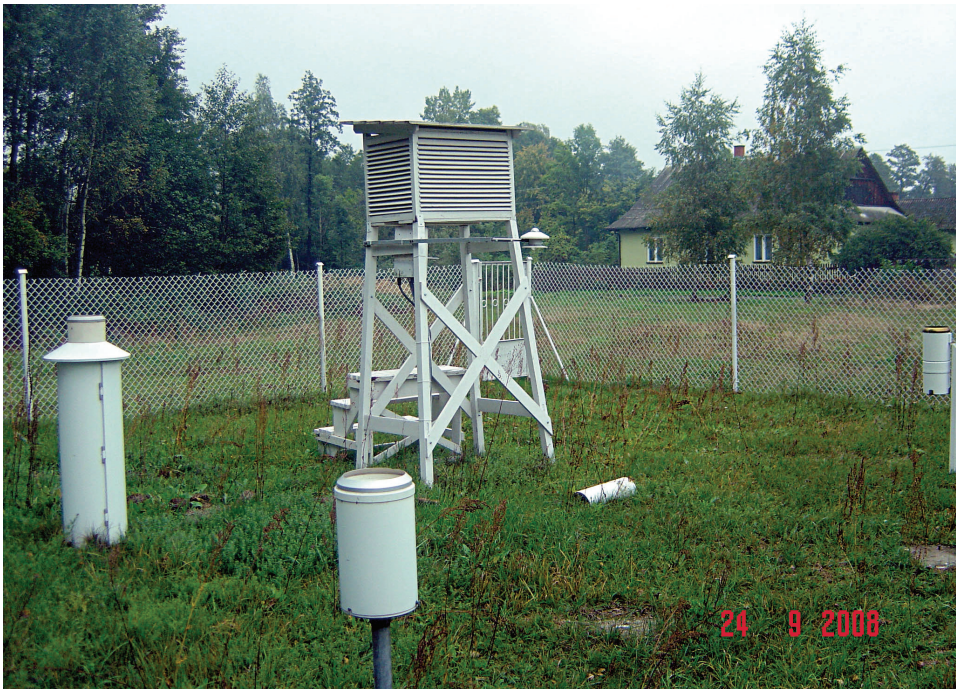
FIGURE 1.3. Meteorological gauging station at Czarna in the Zagożdżonka catchment
